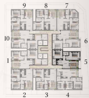
Apartment 5 Northeast-facing Total area: 88.27 m 2
